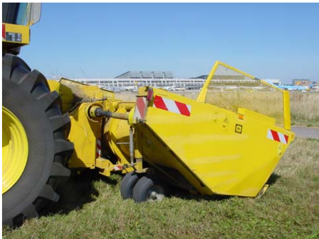
The swivelling wheels of the harvesting unit for the variation of the cutting height from 0 to 35 cm
