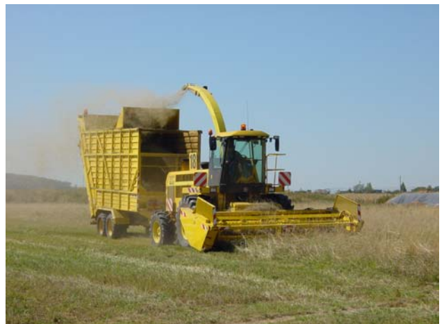
Fig. 3: Mowing and chaffing machine John Deere 6750 with swath container
