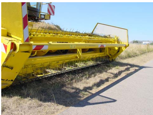
Harvesting unit (field grass cutting unit) with a working width of 420 cm and duplicate cutters
