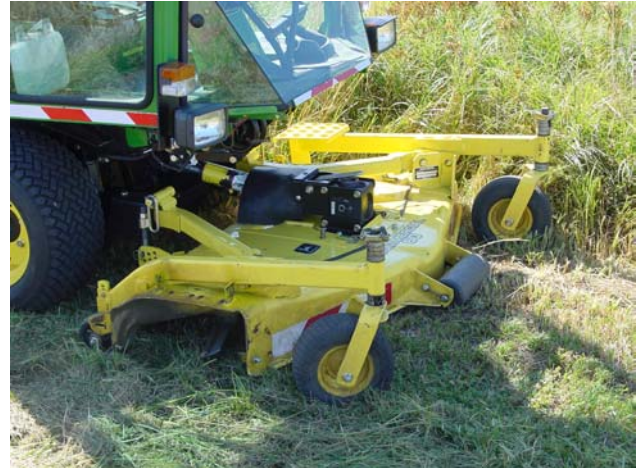
Rotary mower with 1.53-m 3-blade-sickle cutter units with side discharge
