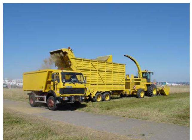
Swath transferred to transport vehicles with container platforms
