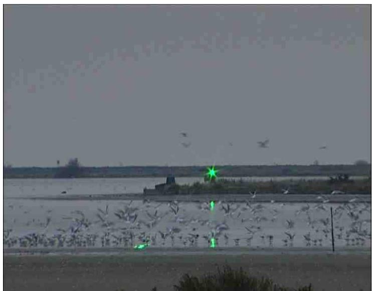
In 2000, a prototype of automatic system scanning the runways with a low low height laser beam is developed in France. The beam's specifications guarantee a complete ocular safety for both ground staff and cabin crew.
