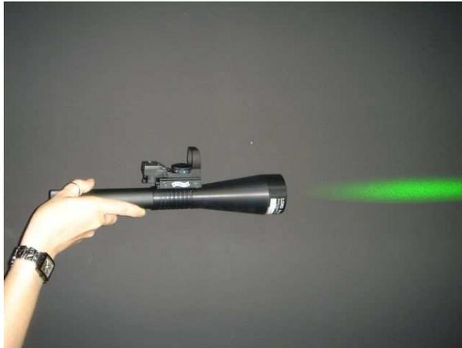
The method consist to approach a green laser on sitting birds in order to get their flying off; range around one kilometer under lighting conditions of less than 13000 lux.
