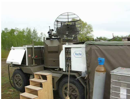
Fig 3: Tracking radar “Superfledermaus” used for validating quantitative measurements by weather radar.
