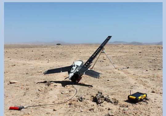
An example of the Gatewing RPA system on its launch rail. Source Wiki Commons
