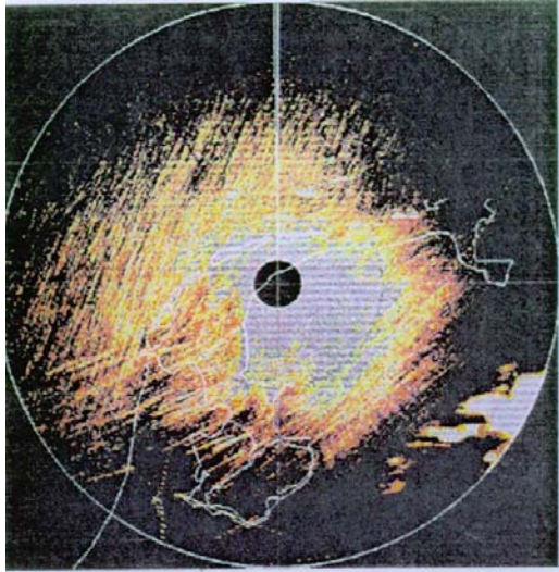
Fig 4. Digital "time exposure photo" of 10 minutes of the radar image of the lowest beam of a stacked beam RNLAf air defence radar. The orange and yellow stripes represent SSW bird movements across the North Sea and SW bird movements across land. Green and blue colors indicate saturation of birddechoes, groundclutter and a rain cloud above the border with Germany. Stippled lines near Amsterdam represent airliners towards or from Schiphol airport.
