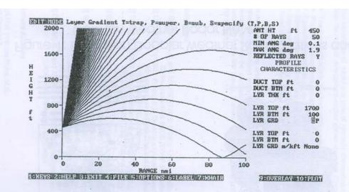
Figure 2: Superrefraction of Radarbeams due to Anomalous Propagation Conditions of the Atmosphere, Causing Ground Clutter and Hight Errors
