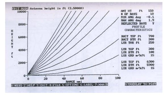
Figure 5: Propagation of Radarbeam According to Atmospheric Conditions over Northern Germany at 11.05.98/06 UTC
