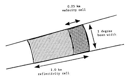
FIGURE 2. Low-height coverage of the NEXRAD beam.
