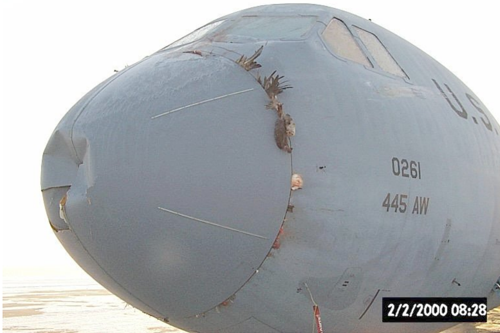
Figure 2. Canada Goose strike on radome of US Air Force C-141.
