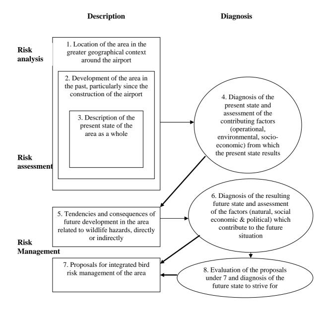
Figure 2: Methodology applied for the integrated bird risk management of the area off the airport of Kavala
