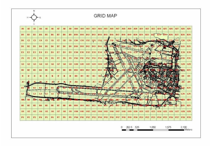
Figure 3. An alphanumeric grid adapted to display ground count data at Dublin Airport in ArcGis.
