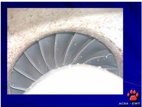
The turbofan blades visible through the engine turbo air intake shows some damage and bird debris is visible all throughout the air intake cowling and inner surface.
