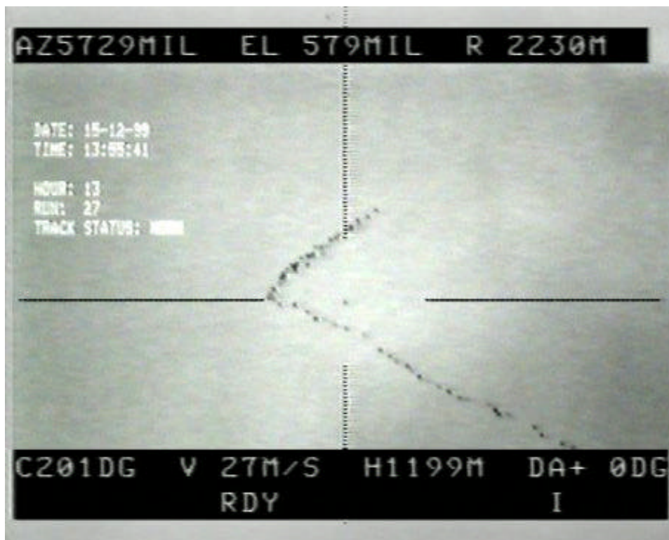
Fig. 3. Picture of migrating goose flock made by tracking radar on 15 December 1999 near IJmuiden. Ground velocity (27 m/s) as well as flight height (1199 metres) are indicated.
